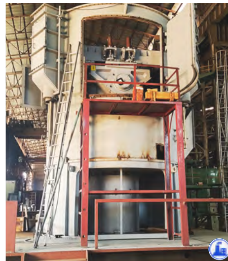
Control Assembly of Coal Pulverizing Mills
